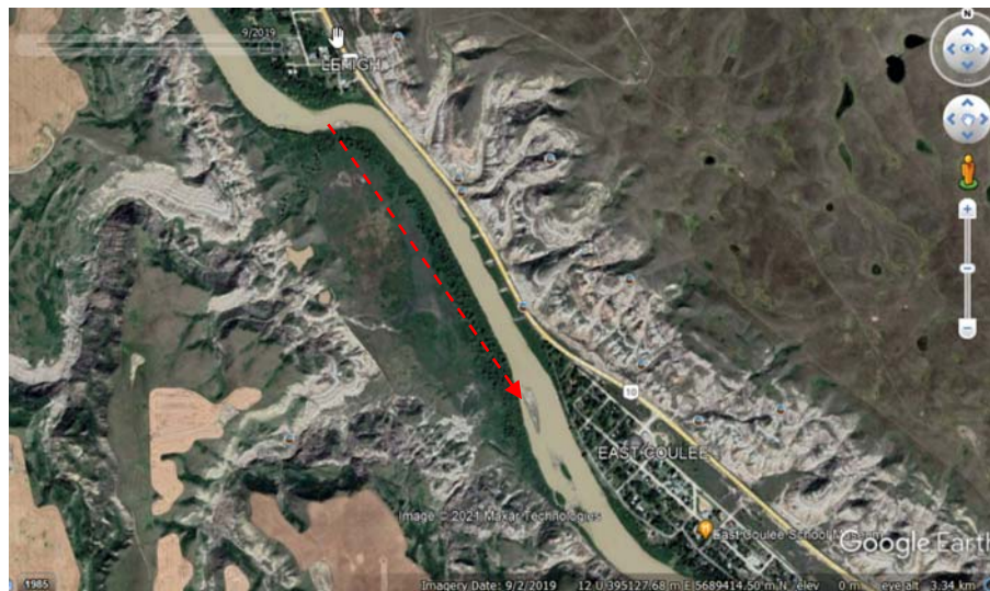
Figure 4-1: Channel Straightening Measure
