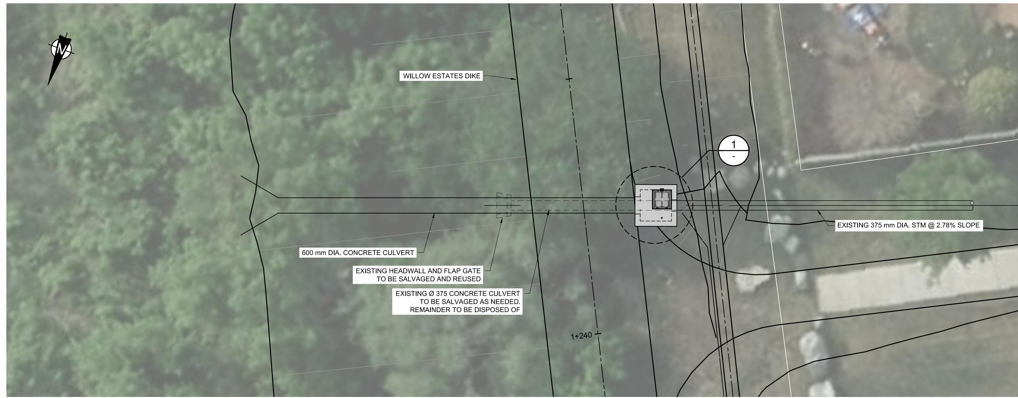
PLAN - CULVERT UPGRADE AT STA 1+246 Scale 1:75
