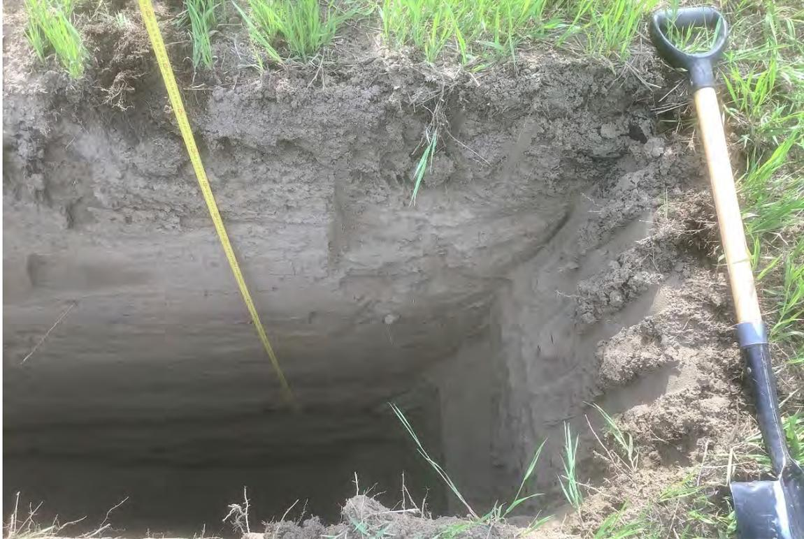
Figure 9. Soil profile of BHT 1 on the floodplain in Target Area 1. The lack of an Ah Horizon, indicating disturbance, is clearly visible.
