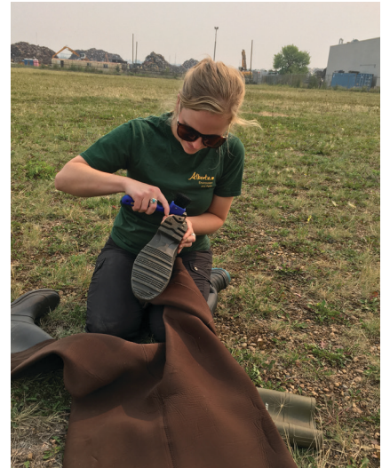
Figure 4: Cleaning waders by manually removing organic debris
