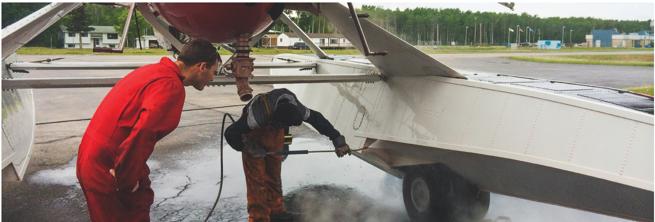
Figure 14: Decontaminating a float plane
