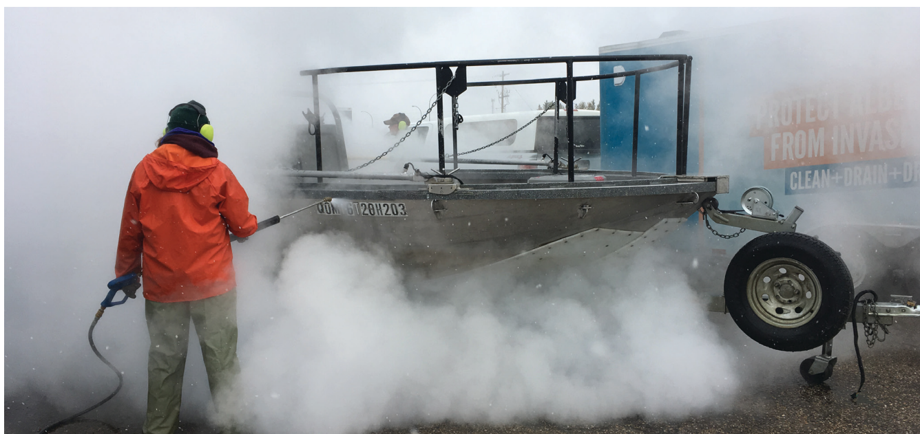
Figure 8: Level 3 Temperature Treatment using Steam
