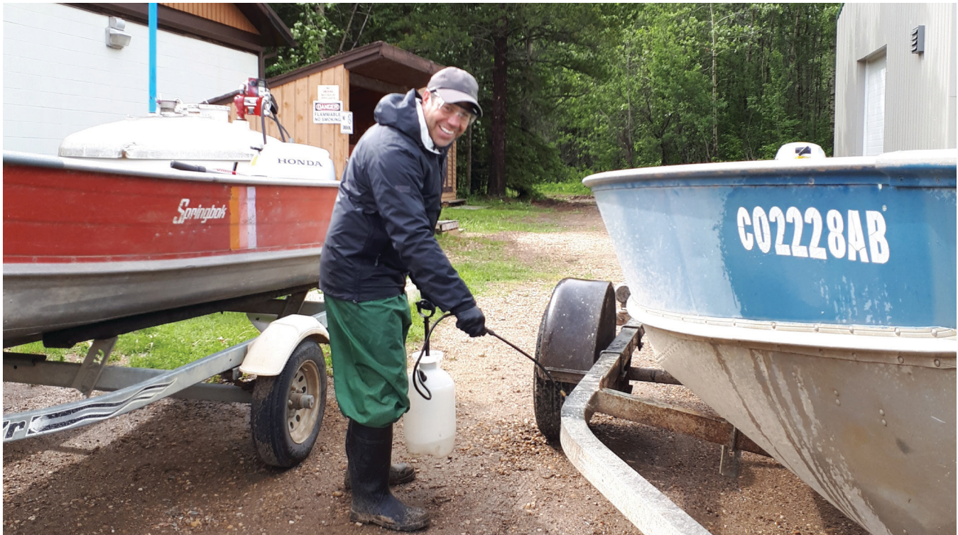
Figure 6: QAC application using a pump-up style sprayer.
